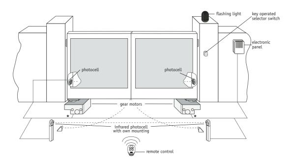
(\*) **CUBIC 6** =  $3 \times 0.75 \text{ mm}^2 + 1 \times 1.5 \text{ mm}^2$ **CUBIC 6H** =  $2 \times 1.5 \text{ mm}^2$
