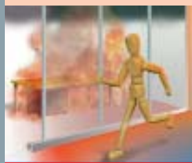
E = Provides a physical barrier against flame, hot toxic gases and smoke
