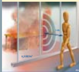
EW – Control of the transmission of radiated heat below a specified level
