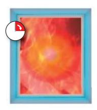
This difference in temperature leads to varying expansion, causing tension of the glass. Normal glass would break immediately from this kind of pressure.
